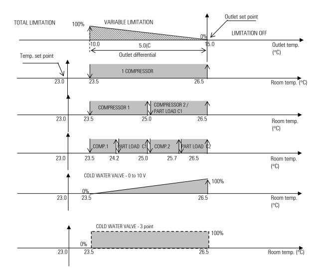
As can be seen, if the outlet temperature is between the outlet set point and the outlet differential, the cooling devices are only partially limited, to a greater extent the lower the temperature.
