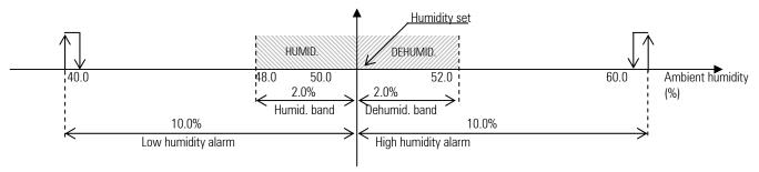
The high and low humidity alarms cause a signal on an alarm screen and have a modifiable delay.
