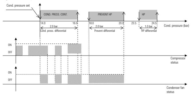
For operation with modulating outputs, refer to the following diagram:
