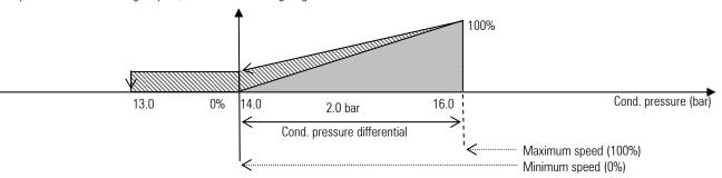
The voltage values corresponding to the minimum and maximum speeds of the fan can be set, between 0 and 10 V; if the minimum value set is greater than 0 V, when stopping the fan is operated at the minimum speed for 1.0 bar below the condensing pressure set point, before switching off, as per the diagram above.
