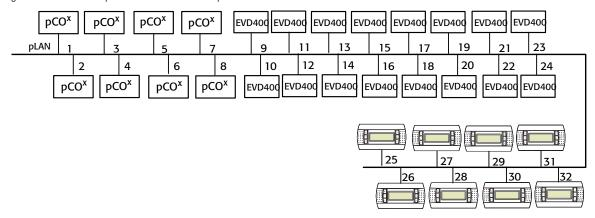
Below is a diagram with the EVD400 driver in a tLAN connection, while the others components are connected in the pLAN:
