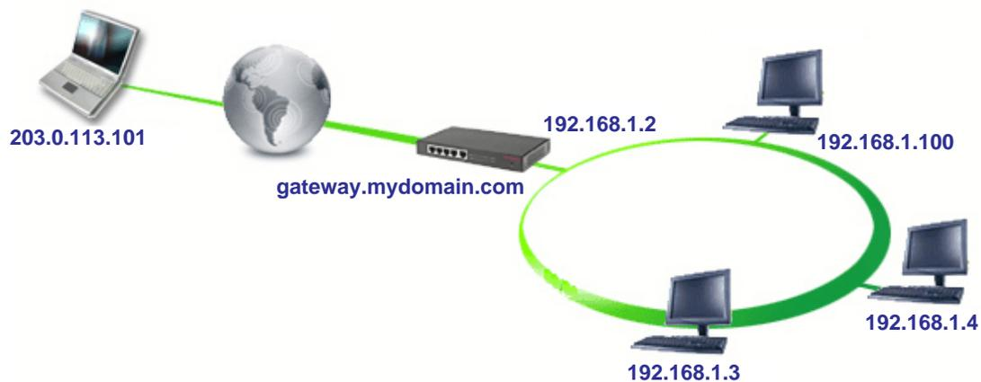
Figure 4. VPN connection between a computer and a remote corporate LAN
