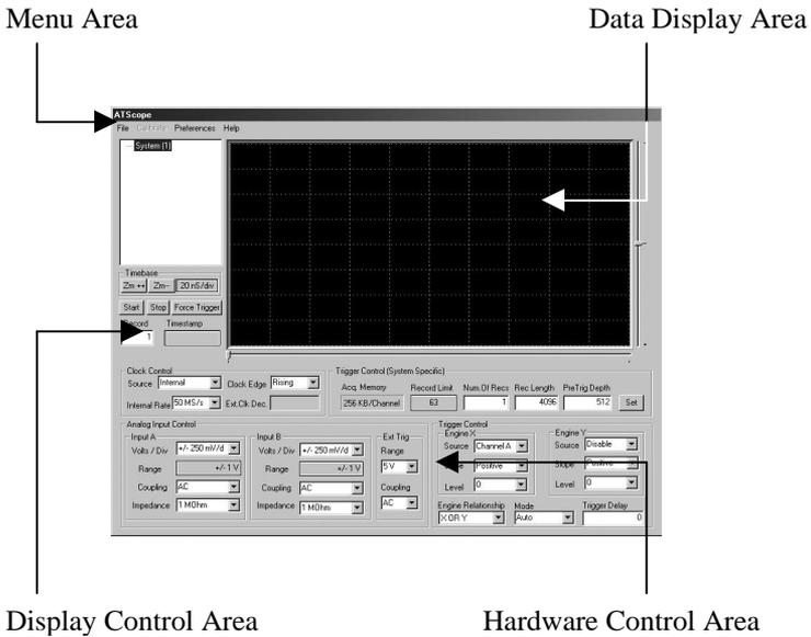
**Data Display Area** is an oscilloscope style grid of 8 vertical and 10 horizontal divisions. There are exactly 256 rows of pixels in the display, allowing 8-bit data to be displayed without any loss of data.
