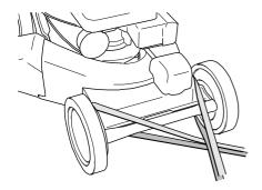
Use tension belts to secure the device.
