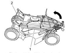
1. Flip the guide bar (1) backwards and engage it with the bar fixing (2).
