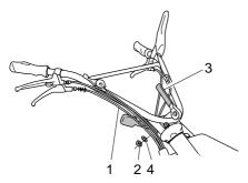
**Attention:** Do not crush the Bowden cables (1) when fixing the handlebar.
