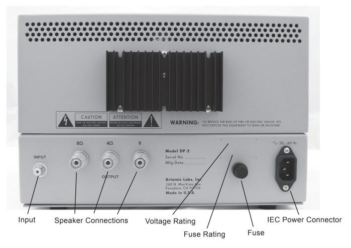
The rear panel of a single channel of the DP-2 amplifier is shown above. Note that the component placement for the two amplifiers are mirror images of each other.
