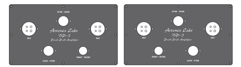
The tube locations are marked on the black plates on the top of the chassis. Note that on both the left and right amplifiers, the two large pins of the 2A3s face right when viewing the front of the chassis, as shown above.
