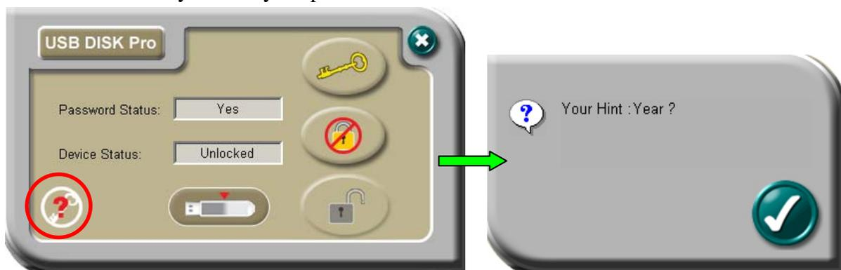
Once you have entered the correct password, the secure partition will be available temporarily until you **remove your device from the USB port** or if there is a suspension in power. You can read and write data to the secure partition once it is unlocked.
