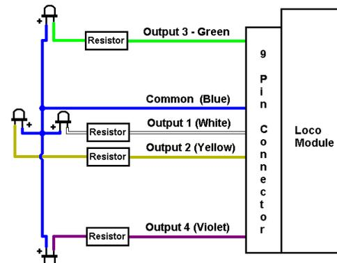
**WARNING:** Using LED's without resistors can damage the LED's! Use 1k Ohm 1/4 W for 15mA or 750 Ohm 1/2W for 20mA.
