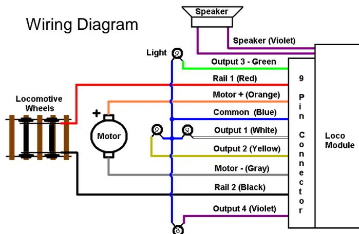
Wiring Diagram using LED's for Lights
