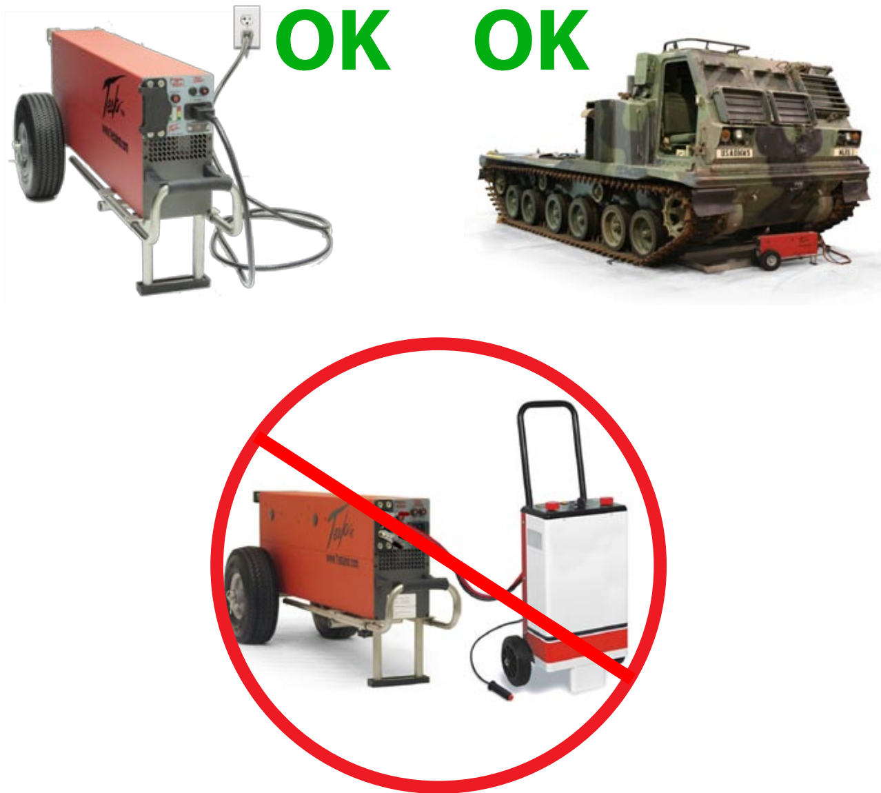
Figure 4.3.3 - Proper and Improper Charging Methods
