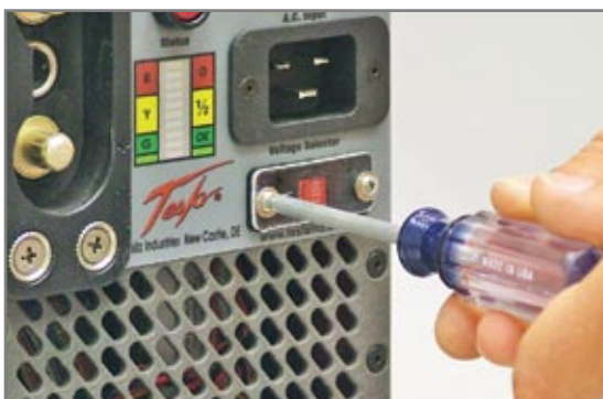
Figure 2.10.2 - Unscrew Protective Cover
