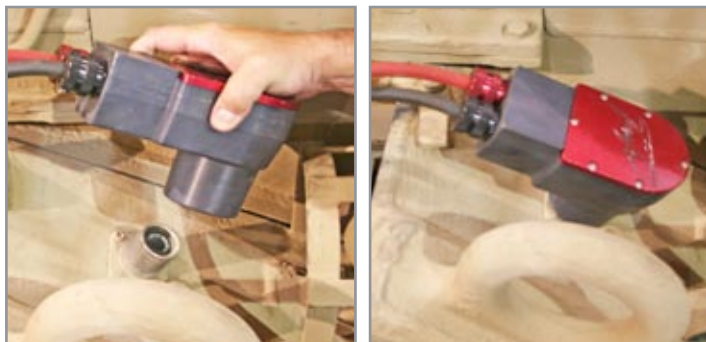
Figure 3.11.2 Attaching NATO DC Power Cable to vehicle
