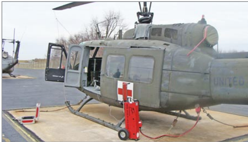
Figure 3.11.4 Starting UH-1 Huey Helicopter with TI2000 GPU-24
