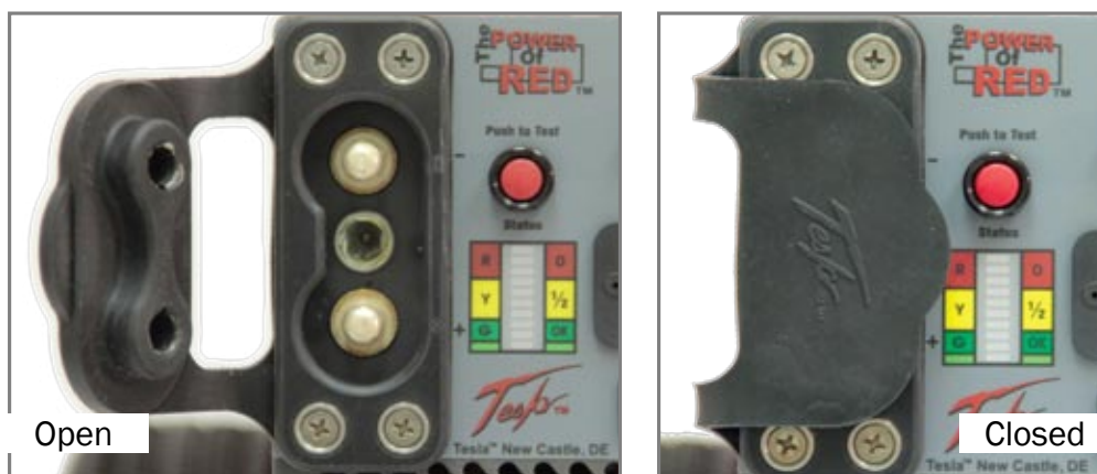
Figure 2.9.1 - 24 VDC Output Connector Protective Cover
