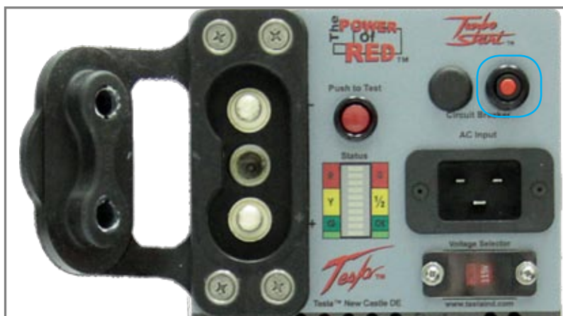
Figure 2.8.1 - AC Input Circuit Breaker (outlined in blue)
