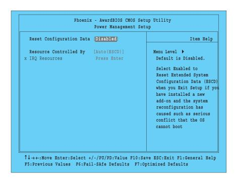
This section describes the configuring of the PCI bus system. PCI, or Personal Computer Interconnect, is a system which allows I/O devices to operate at speeds nearing the speed the CPU itself uses when communicating with its own special components.
