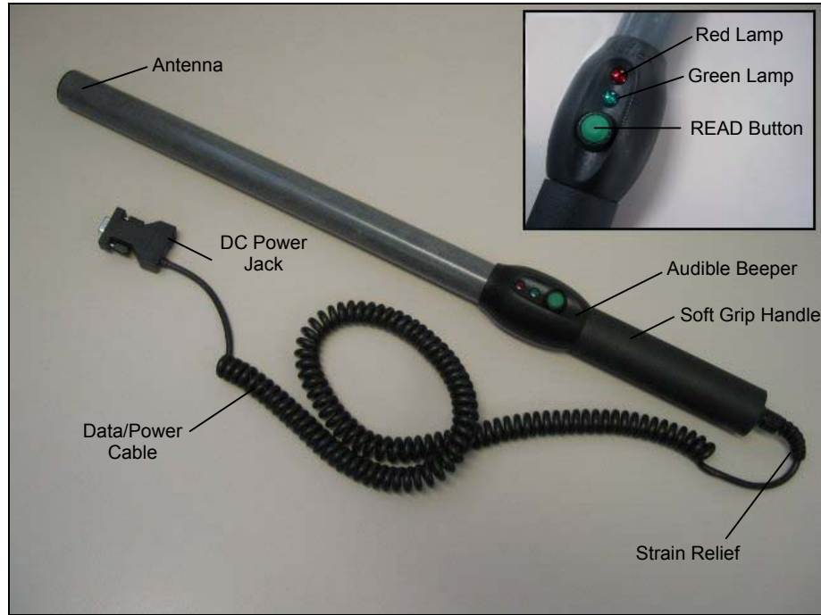
Figure 3 – Features of The Allflex Stick Reader
