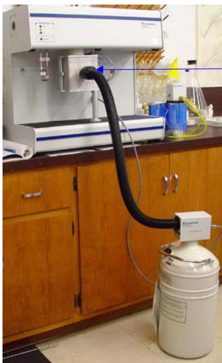
Delivery hose connection (tighten thumbwheel to secure)
