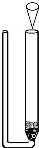
Figure 4-11. Sealing the Sample Tube
