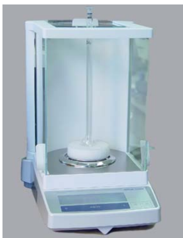
Figure 4-9. Weighing the Sample Tube
