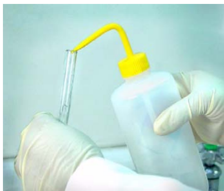
Figure 4-6. Rinsing the Sample Tube
