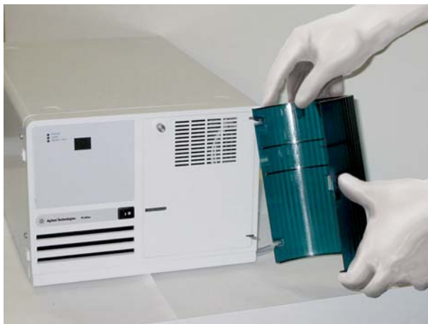
Figure 17 Installing the Agilent 325 Detector door
