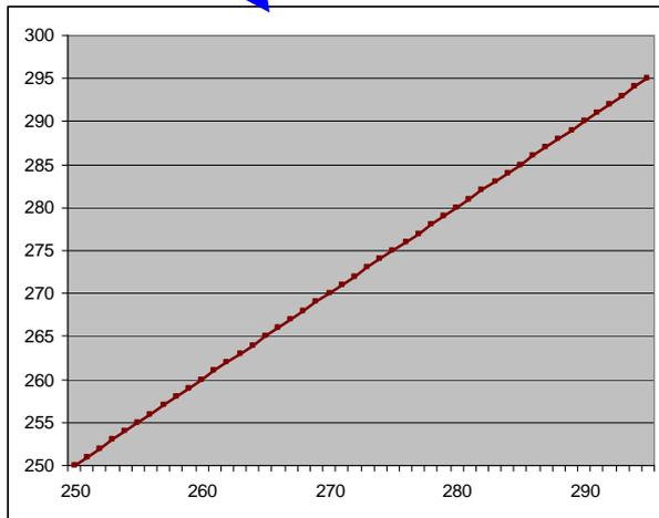
An increment of 1 LSB is made for each pixel. When it reaches 4095, turns back to 0 and starts again
