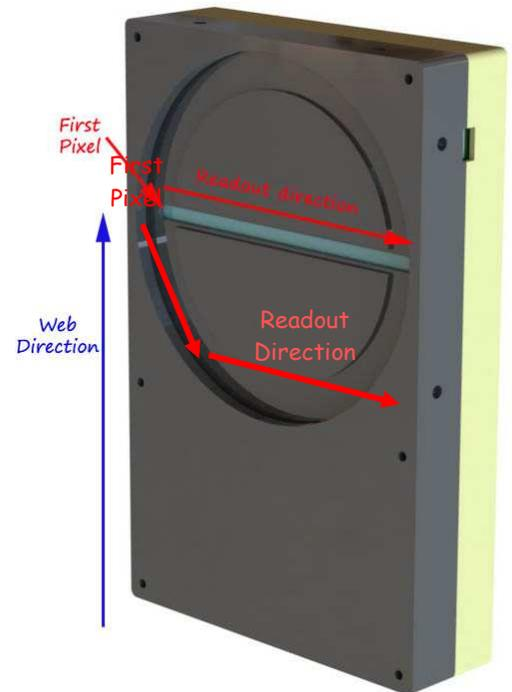
This positioning takes also in account that the mode "Reverse X" is "Off" (Normal readout direction)
