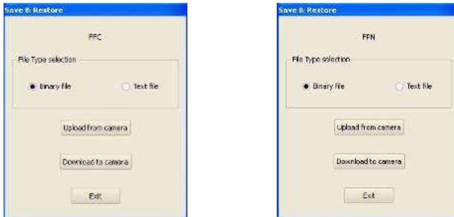
This will allow the user to upload/download out/in the Camera the FFC coefficients in/from a binary or text file that can be processed externally.
