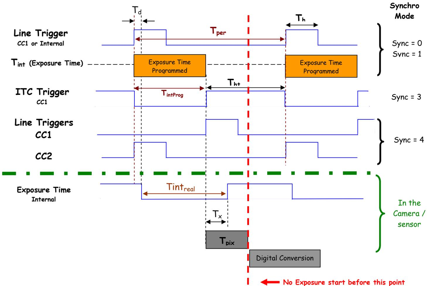
$T_{pix}$  : Timing Pixel. During this uncompressible period, the pixel and its black reference are read out to the Digital converter. During the first half of this timing pixel (read out of the black reference), we can consider that the exposure is still active.
