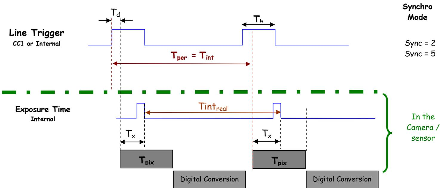
In these modes, the rising edge of the Trigger (internal or External) starts the readout process ( $T_{pix}$ ) of the previous integration. The Real exposure time ( $T_{int_{real}}$ ) is finally equal to the Line Period ( $T_{per}$ ) even if it's delayed from ( $T_x + T_d$ ) from the rising edge of the incoming Line Trigger.
