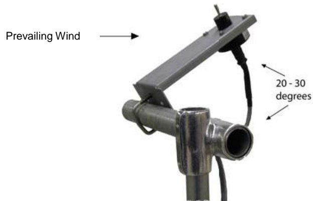
Figure 4 Mounting (part #0871LH1 MNT)
