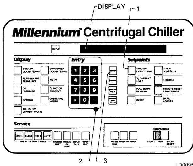
**FIG. 6 – KEYPAD – PROGRAMMING “LEAVING CHILLED WATER TEMP” SETPOINT**
