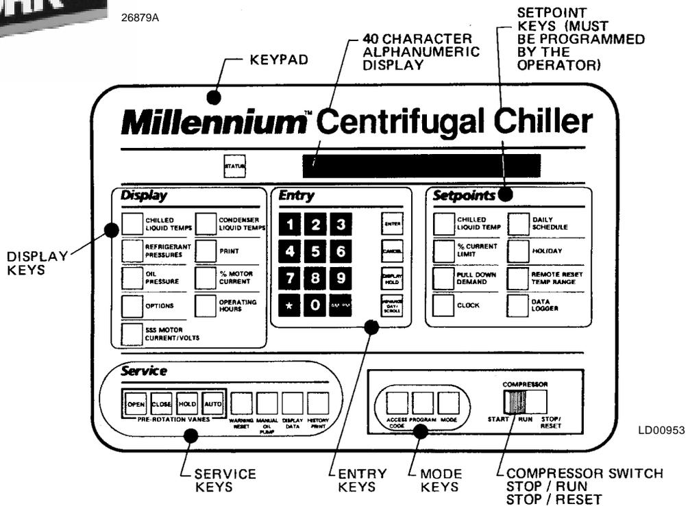
**FIG. 3 – MICROCOMPUTER CONTROL CENTER AND KEYPAD**
