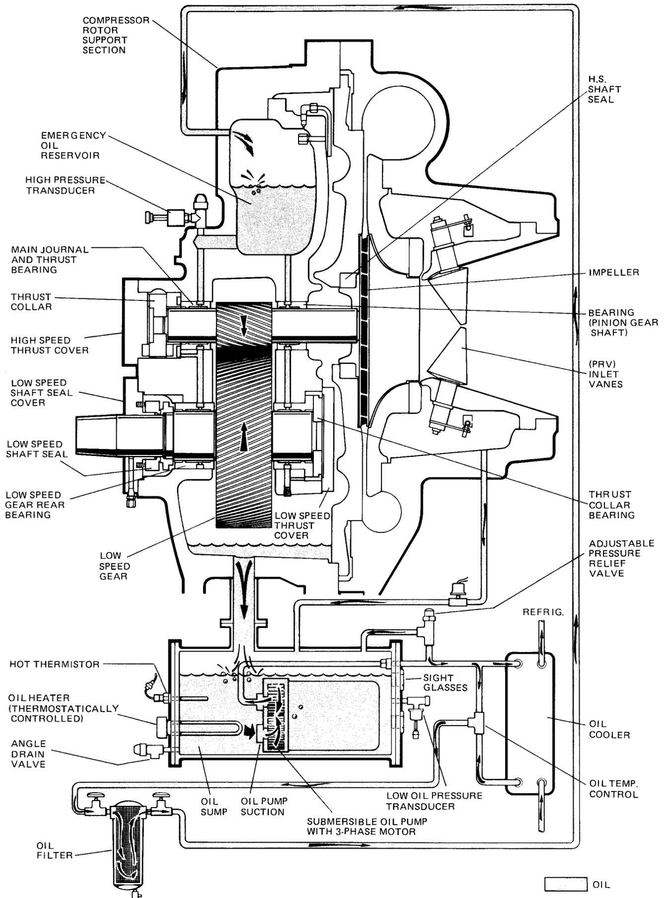
FIG. 18 - SCHEMATIC DRAWING - (YK) COMPRESSOR LUBRICATION SYSTEM
