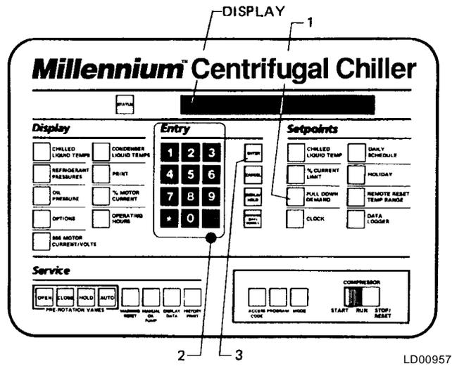
**FIG. 8 – KEYPAD – PROGRAMMING “PULL DOWN DEMAND” SETPOINT**
