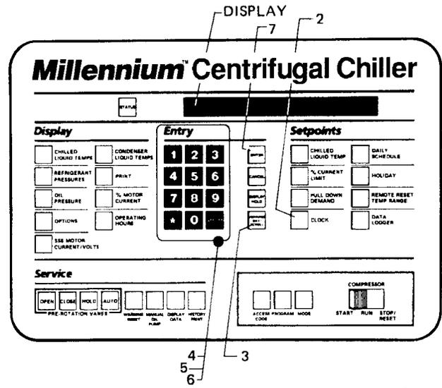
**FIG. 9 – KEYPAD – PROGRAMMING “CLOCK” SETPOINT**
