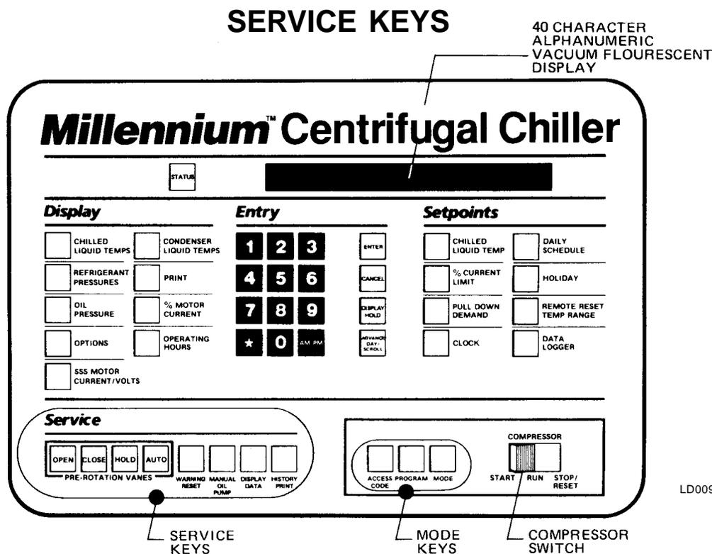
FIG. 13 – KEYPAD – SERVICE KEYS LOCATION
