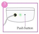
Start the treatment program simply by pressing the button. The LED indicator will light up green. The therapy will stop automatically after 5 minutes.
