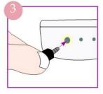
Plug the connecting cable from the LED holders into the socket on the front of the unit.
