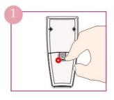
Unlatch the lid on the back of the unit, fold it up and remove.
