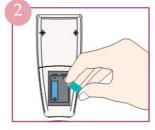
Insert the batteries, put the lid back in position and latch it in place.
