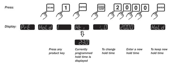
**NOTE:** Up to 4 hold timers can be programmed per product key on the 8 button controller; up to 8 hold timers can be programmed per product key on the 16 button controller.
