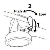
The cutting height adjustment lever is situated above the right rear wheel. To adjust the cutting height, pull the height adjustment lever out and away from the lawnmower and move forward or backwards into another slot depending whether you want it to cut shorter (low) or longer (high).
