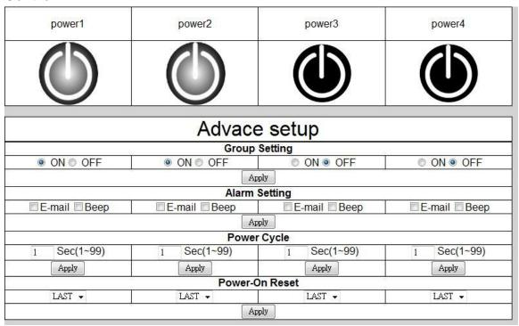
The Power Controls page allows you to setup the name of each port, control each power or all the 4 powers ,ON / OFF enable alarm as outlet status change , and also the power status as Reboot.
