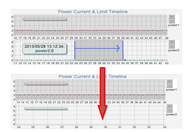
B-4 As mouse move to the line chart, there is message board shows time, current and consumed power current in a square as following:
