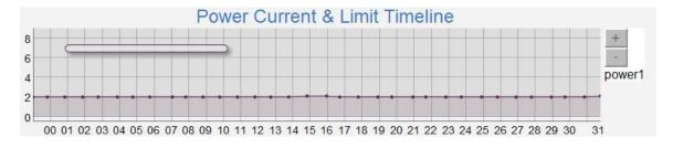
B-2 User can adjust the Current display range by pressing the +/- button at right side as following: .
