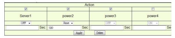
• Enable section: Select the power to activate as ping fails by the mark "v" in the small box
