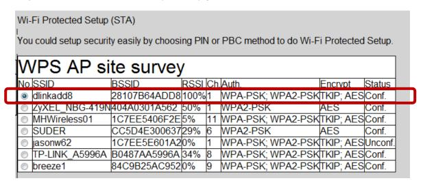
Step 2: Select Mode "Enrollee" and press "PBC Start" and then press the WPS buttons on WIFI AP (Router) soon in few seconds.
