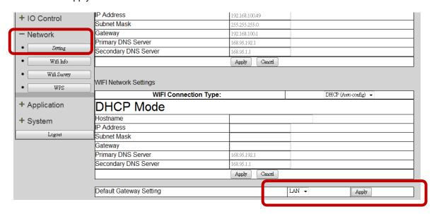
Step 3 : Connect your PC and 9258W2 to a router by LAN. Then  $\bf reboot$  9258W2 (MUST  $\bf DO$ ) . After 45 seconds with a long beep, you can found the LAN IP of 9258W2 by IPEIDT.exe
