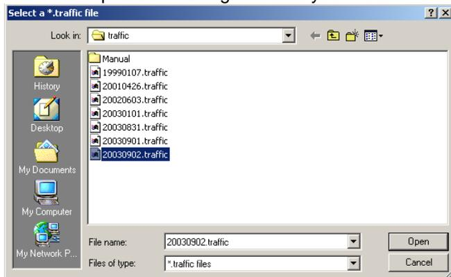
Select the desired file and click the **open** button. Then the software will start extracting the detector list and build a table. After the detectors are loaded a message box will appear on the screen prompting the user that the loading of data has been completed. Click OK to proceed.
