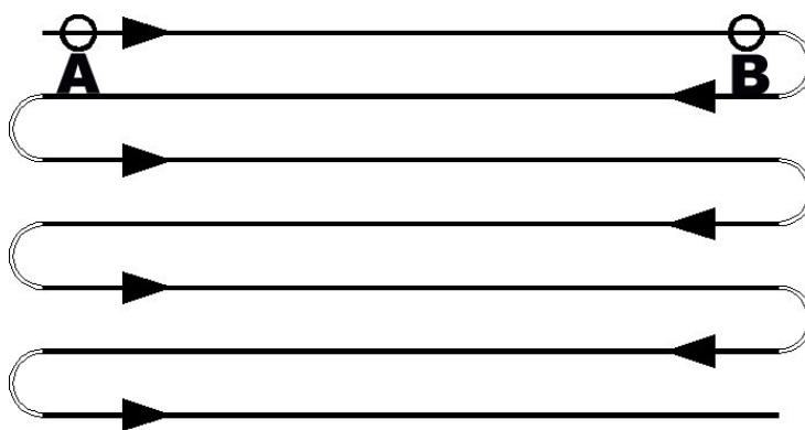
Figure 5-4: A typical spray pattern using parallel guidance. Points “A” and “B” define the base line for all other parallel lines.
