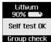
While starting, the device conducts a selftest. If the self-test fails, an error message is displayed for 20 seconds along with an acoustic warning. If the battery power falls below 20% or the battery icon is displayed, the batteries must be replaced as soon as possible!
