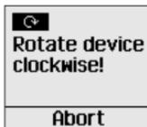
ceiver slowly and with constant speed clockwise until the message «Device calibrated!» appears.
