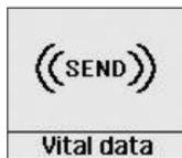
The SEND mode is the normal operating mode outdoors or in all other situations in which there is a risk of avalanches. Each time the SEND mode has been activated, this is confirmed by a triple beep sound. Each individual signal pulse is tested. If the test is successful, this is confirmed by a blink of the red SEND-Control LED. The LCD display is automatically deactivated in the SEND mode
