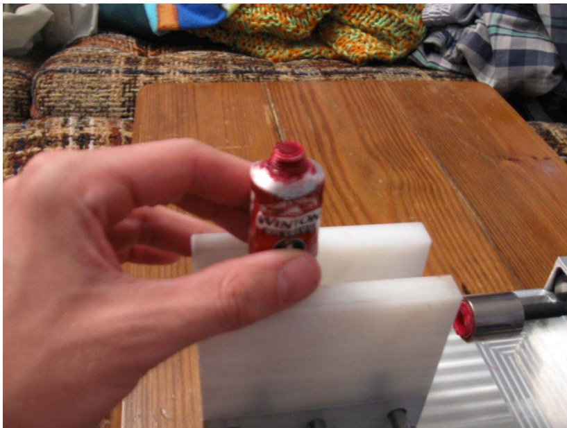
11) Slide paint tube into vise vertically, with threads on top
