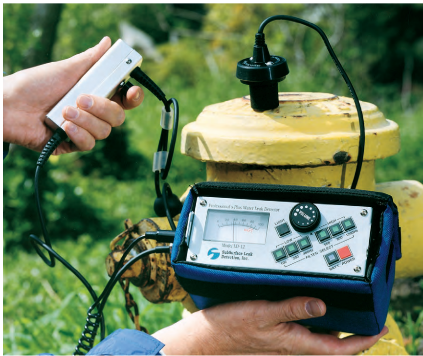
Figure 4-6 Leak Survey at a Hydrant
