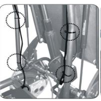
4. Please use the cable tie to fix it. The cables should be fixed inside of the two tubes
