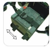
36AH Battery fixing direction.
