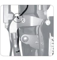
2. To pack the chair into 3. Please note the a carton, the circled place is not fastened by the cable tie. Please fasten it with a cable tie as soon as you unpack the chair
