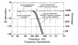
Recently there has been increased use of power through inverters. switching regulators, etc. When the high frequency noise from such appliances leaks or flows into the ground through capacitors not filtering completely, the earth leakage breaker may trip even though there is no "actual" leakage. In such a case, the instrument do not give leakage current reading if "50/60Hz" frequency response is se-Take care readings with the 50/60Hz and WIDE frequency responses
