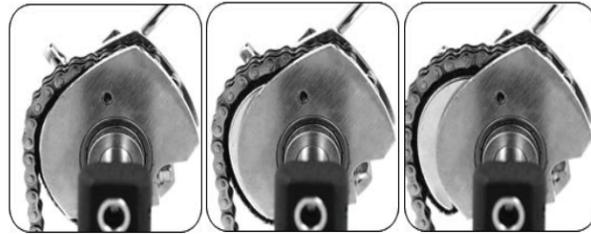
Torque position adjustments from eccentric (far left) to concentric (far right).
