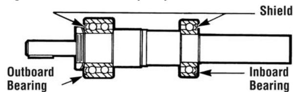
Figure 5-8: In-Line pump shield orientation
