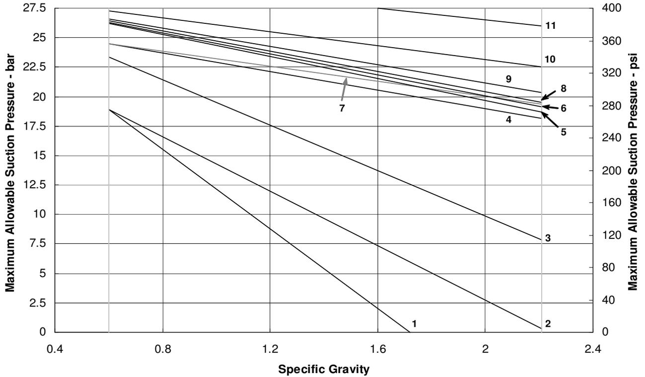
Figure 3-5b: Suction pressure limits 3 500 r/min
