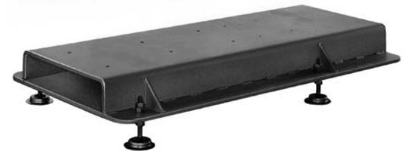
Baseplates intended for grouted installation are designed to use the grout as a stiffening member. Stilt mounted baseplates, on the other hand, are designed to provide their own rigidity. Therefore the designs of the two baseplates are usually different.
