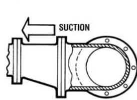
Avoid the use of throttling valves and strainers in the suction line. Start up strainers must be removed shortly before start up. When the pump is installed below the source of supply, a valve should be installed in the suction line to isolate the pump and permit pump inspection and maintenance. However, never place a valve directly on the suction nozzle of the pump.
