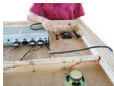
FIG-15 Push down the wires into the room
