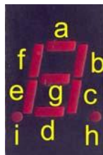
Figure 1. A Seven-Segment Display
