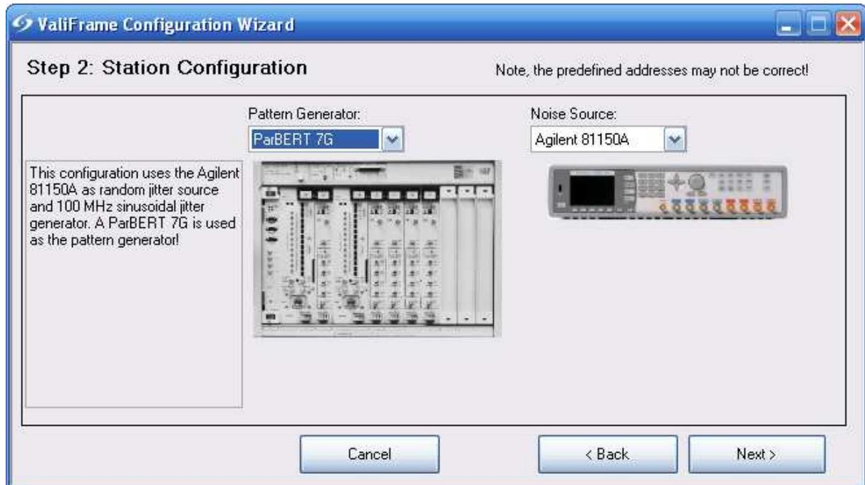
Figure 3 Selection of the Station Setup
