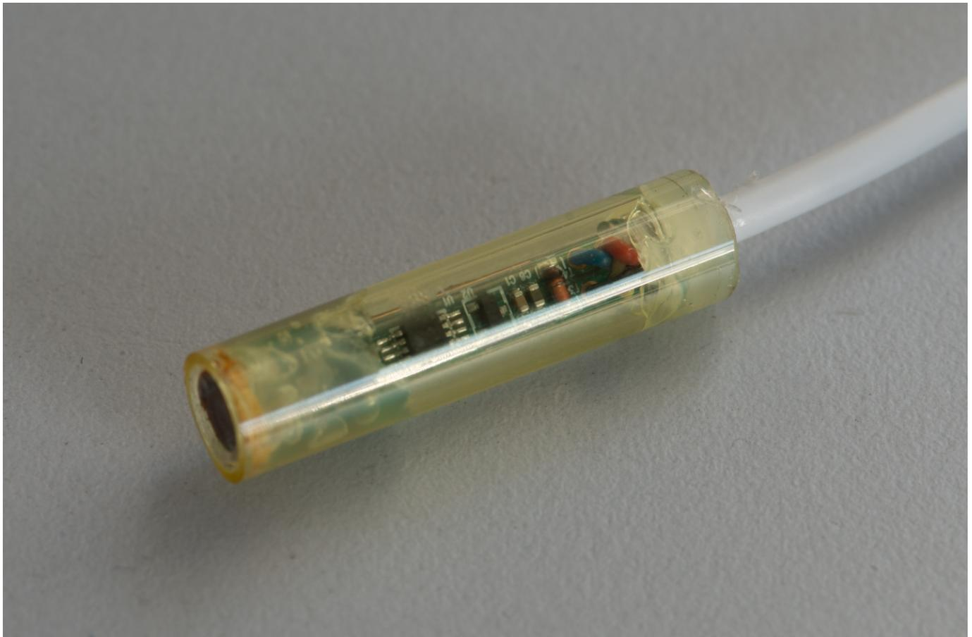
**Figure 63.** *BudkaLTS* board closed in a cover.
