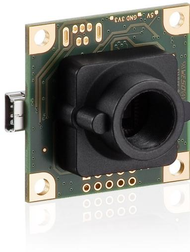
**Figure 8.** Photo of the *UI-1541LE* monochrome industrial camera. From [11].
