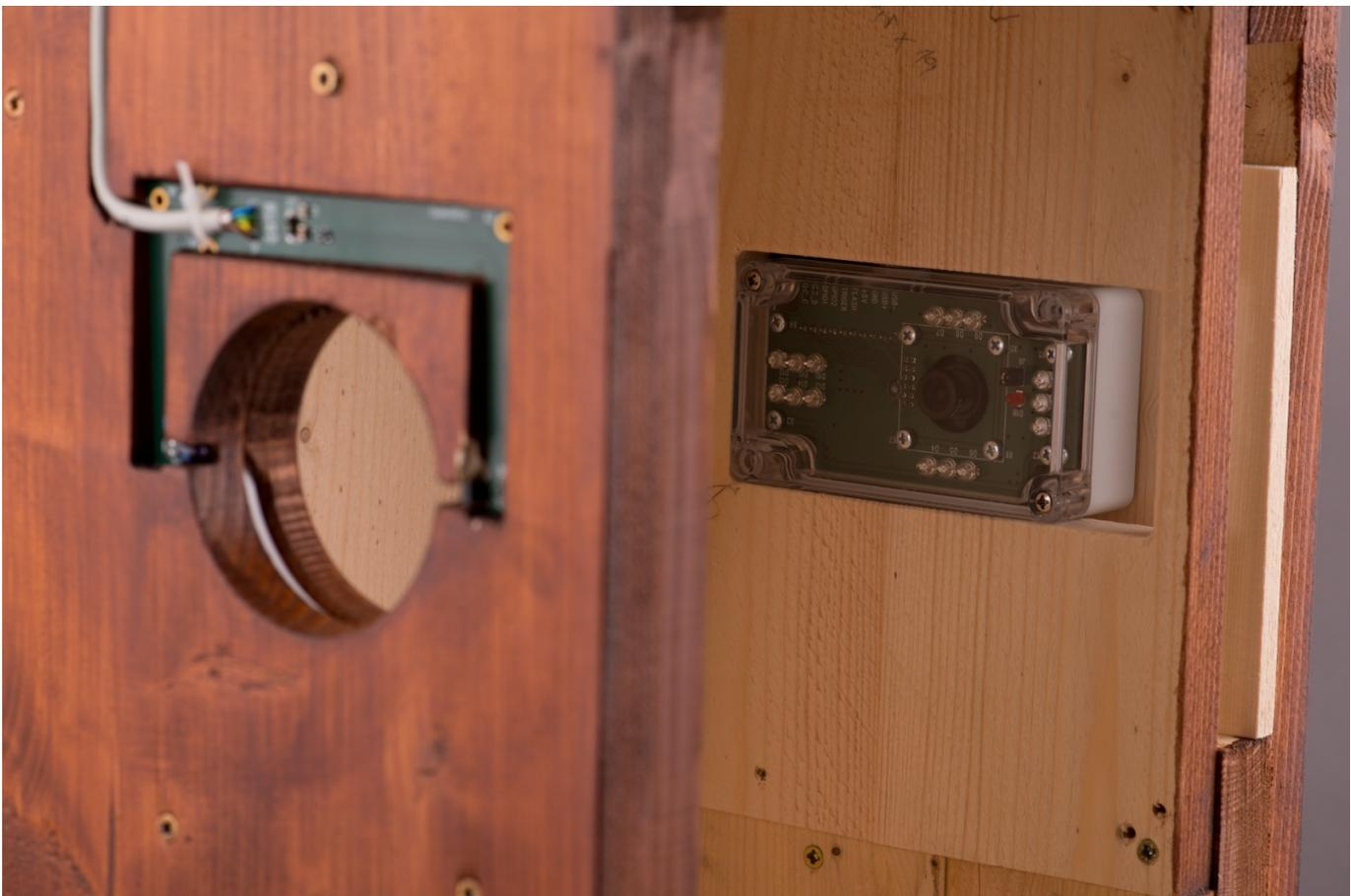
**Figure 65.** Installed *fly-in* camera, light barrier and RFID antenna.
