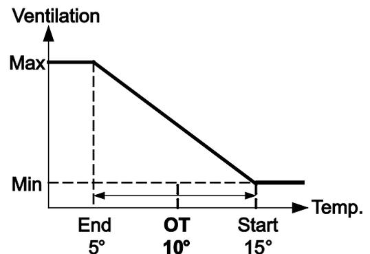
The settings low outside temperature *Start*, low outside temperature *End* and *Influence factor* determine the bandwidth increase. The control computer calculates a *Bandwidth* from these three settings. The *Bandwidth* increase is as follows:
