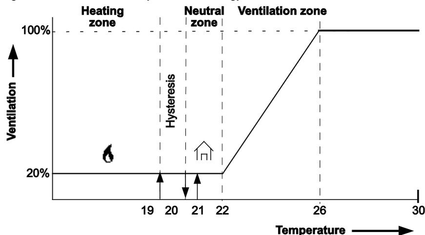
Figure 2: Ventilation graph. Setpoint house is 21°C, the control value heating is 20.5°C.
