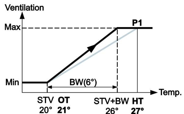
If the outside temperature falls (greatly) the cold air will also cause the house temperature to drop. The control computer will control using a lower ventilation position after point **P1** has been reached. The example shows the ventilation position at a house temperature of 25°C.
