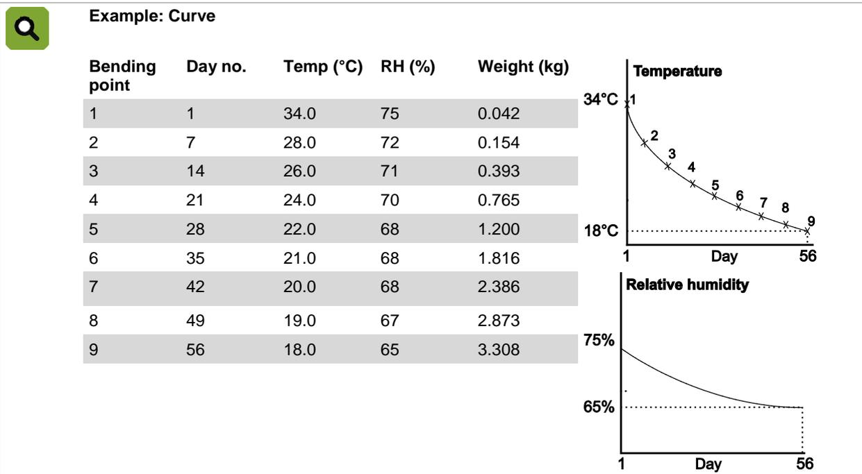
The bending points of the curves can be entered in the screen below.
