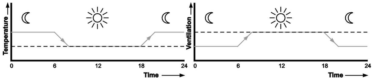
When night correction is active, the control computer adjusts the setpoints of the house temperature and the minimum ventilation accordingly. If the light level of the linked light clock gradually increases or decreases, these setpoints are adjusted accordingly.
