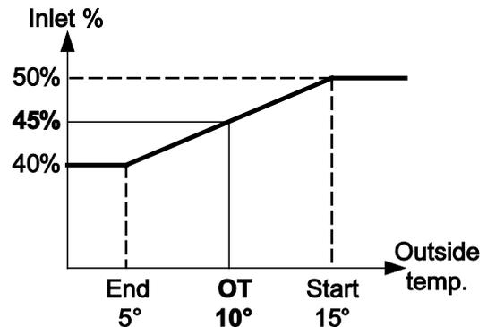
The factor influence is 0.8. The *Control value air / extra inlet* can therefore be lowered to  $0.8 \times 50\% = 40\%$ . The actual outside temperature is 10°C, precisely midway in the influence path. The *control value air/extra inlet* is then 45%.
