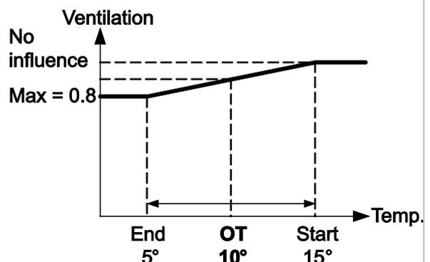
The settings low outside temperature *Start*, low outside temperature *End* and *Influence factor* determine the minimum ventilation setpoint decrease. The control computer calculates a new *Setpoint minimum ventilation* from these settings. The new setpoint is calculated as follows:
