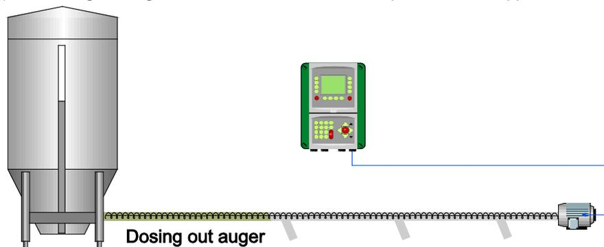
3. The hoppers are filled successively according to the overflow principle. When the last hopper is full (detected by the demand sensor), the control computer stops supplying feed.
