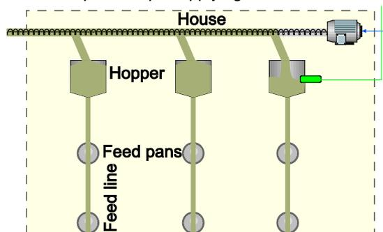
4. From the hoppers the feed line augers transport feed to the feed pans. The feed pans are also filled according to the overflow principle.
