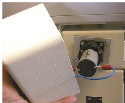
Figure 6-6 Width motor wires
