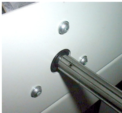
Figure 6-2 Screws and shaft pin
