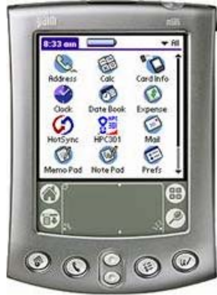
Figure 3.1 - Smar's HPC301 Hand-Held Terminal
