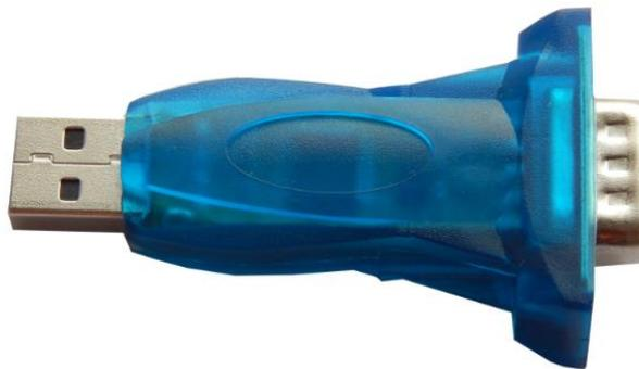
**Note:** We do not support the 3rd party USB-RS232 adapters, even though they might work sometime. The problem is that those consumer electronics rated USB adapters only works in a noise-free environments. This means, once the engine is running, it
