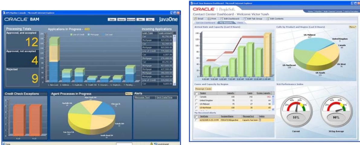
Oracle BPEL Process Manager integrates easily with Oracle BAM. For example, the BPEL Designer includes support for “sensors” which make it easy to push events from BPEL processes out to the BAM server. However, the BAM server can gather events from any source within the enterprise (JMS messages, DB events, etc) that can write to a JMS queue and is not limited to BPEL process events.
