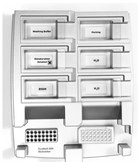
Figure 2. Placement of PCR plate (or strips) and PyroMark Q24 plate on the vacuum workstation.
