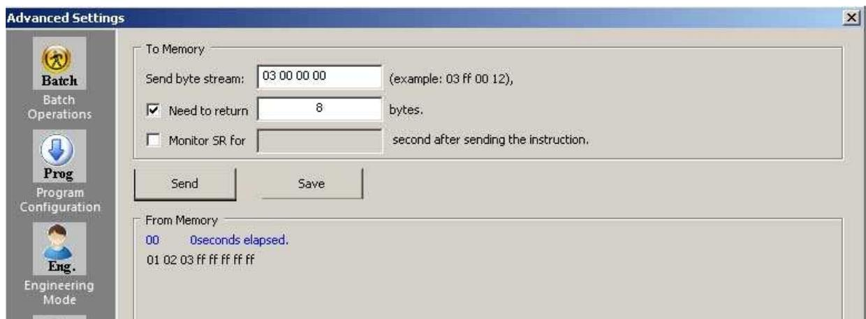
The return bytes from the SPI Flash are displayed in the “from SPI Flash” window: “01 02 03 FF FF FF FF FF”.
