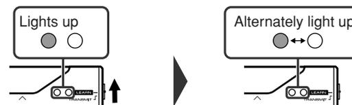
**2 Press the ON/⏻ (STAND-BY) and CLEAR buttons simultaneously for more than 3 seconds.**
