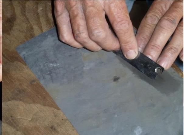
4. Polish the bevel & remove any remaining burr with 1200 grit wet/dry sandpaper. Rub the flat back of the blade once to finish.
