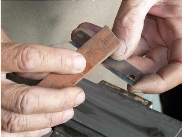
3. ...a fine flat diamond file or small wet stone. Sharpen only the bevel side of the blade. The tip bevel should be no greater than 15°.
