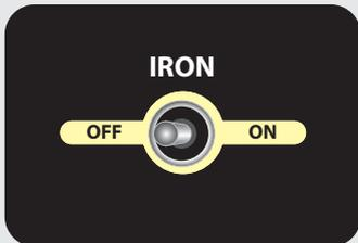
When you want to avoid detecting ferrous metals you can turn the iron switch off and enable the device to eliminate these metals and not produce a warning tone.
