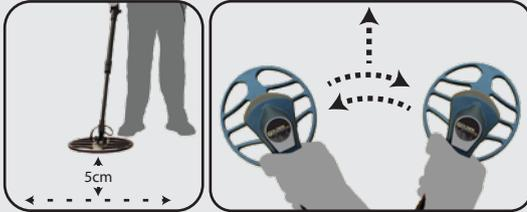
After the settings are adjusted, you can start searching by lifting the search coil 5cm. above the ground and sweeping it right and left, keeping it parallel to the ground.
