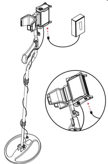
Plug the battery cable into the battery input socket underneath the system box and tighten securely.
