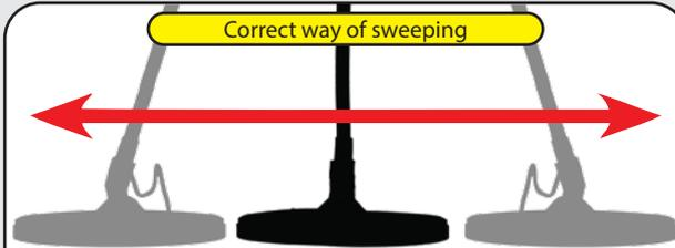
The search coil must be parallel to the ground at all times.
