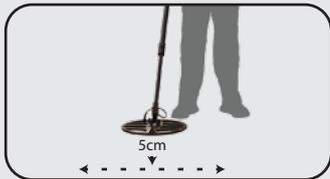
To ground balance, holding the search coil 5cm. above the ground, sweep it right and left, keeping it parallel to the ground and slowly turn the ground balance knob clockwise until the noise is gone and the device is silent. If you cannot ground balance the detector, gradually decrease the sensitivity and repeat the above steps.
