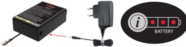
To charge the battery, insert the power cable jack into the socket on the side of the battery and plug the power cable into a 110/220 Volt wall outlet. The LED on the charger will light up red while charging. When charging is complete, it will turn green. This LED will also light up green if the charger is plugged into an outlet without the battery installed in it.
