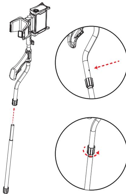
Again by holding the metal pin pressed, insert the upper shaft into the S-rod and click the pin into its hole. Then, secure it by tightening the twist lock.
