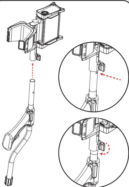
Holding the metal pin pressed, insert the S-rod into its place underneath the system box and secure it by tightening the wingnut as shown in the picture.
