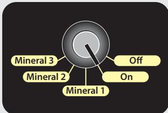
To turn on the device, rotate the On/Off knob to ON. Turn the same knob to OFF position when you want to turn off the device. When the device is turned on, a melody will be heard and approximately 10 seconds later you will hear a long beep indicating that the device is ready to use.
