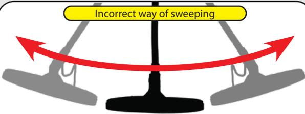
It is important to keep the search coil parallel to the ground in order to get accurate results.
