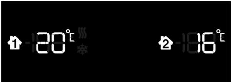
The Solo II has one built-in sensor that is displayed on the left. If the temperature of your home is higher than the temperature you set on the display, the display will show the heatwave icon (SSS). If the temperature is lower, the display will show the snowflake icon (❄). You can purchase an additional sensor that you can pair to the second slot on the right.
