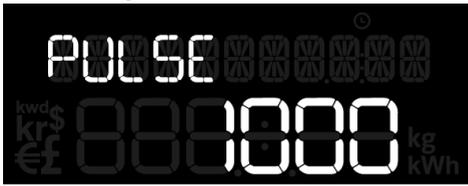
You need to tell the **display** about your electricity meter. The **display** works by detecting the LED flashing on the meter, but it needs to be told how many times the pulse flashes per kWh of energy consumption. This is normally written on the front of your meter e.g. '1000 imp/kWh'.
