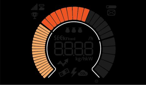
The speedometer shows you how much electricity you are consuming or generating right now depending on which mode you have selected. The **display** refreshes automatically every three seconds.
