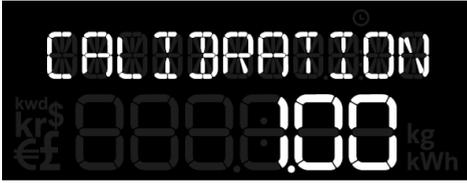
The calibration factor is an advanced setting that typically won't need to be adjusted. Calibration adjusts the accuracy with which the load is measured and the default is 1.00. During normal usage this won't need to be changed.
