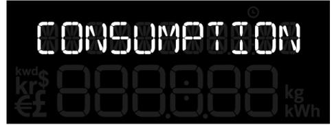
You can use the **display** to monitor your energy use [CONSUMPTION] or generated energy [MICRO-GEN]. The default is [CONSUMPTION] mode.
