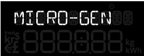
You can use the **display** to monitor your energy use [CONSUMPTION] or generated energy [MICRO-GEN]. The default is [CONSUMPTION] mode.
