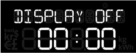
The sleep mode allows you to tell the **display** to turn off overnight. This is done by entering the [DISPLAY OFF] time and the [DISPLAY ON] time. During this time the backlight of the **display** will be turned off – if you want to see the **display** whilst it is asleep simply press any button and it will wake up for 60 seconds. If you don't want to use the sleep mode then you can set it to OFF.
