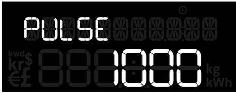
You need to tell the **display** about your generation meter. The **display** works by detecting the LED flashing on the meter, but it needs to be told how many times the pulse flashes per kWh of energy generated. This is normally written on the front of your meter, e.g. '1000 imp/kWh'.
