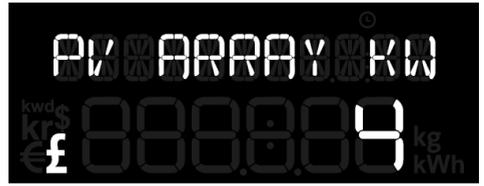
You will be prompted to put in the maximum power that you expect to generate. This tells the **display** the correct range to show on the speed. You can set it to 2, 4, 6, 8 or 20kW by using the ◀ and ▶ buttons and pressing
