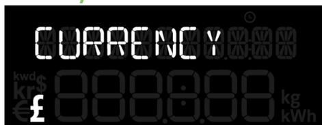
Using the ◀ and ▶ buttons select the £ symbol and press
