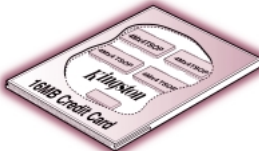
On the surface, credit card memory does not resemble a typical memory module configuration. However, on the inside you will find standard TSOP memory chips.
