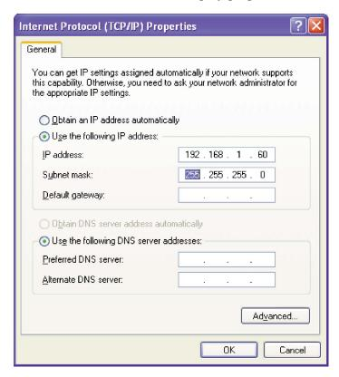
Step 5: Before making any changes to the network settings, write down the current settings (or screen capture the page and print) so that they can be restored once the unit is configured. Next, select the radio button labeled "Use the following IP address" and type in the IP address 192.168.1.60. Type in the subnet mask of 255.255.255.0. Leave the default gateway field blank. Click OK to apply the new settings.
