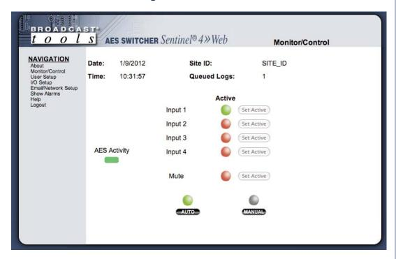
The Monitor/Control page indicates switch position, switching mode, and AES activity. Control of these functions is limited to users with "admin" level access. NOTE: The user defined Site ID, Time, Date and Queued Logs are always displayed. Only "admin" level access can edit some of these items.
