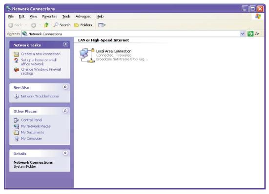
Step 3: Right click on the icon labeled Local Area Connection. Another menu will appear. Select the option at the bottom of the menu labeled Properties. The Local Area Connection Properties window will appear.
