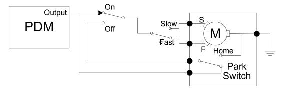
The wiper unit can be wired in a simple two switch arrangement; one switch for power and the other to select fast or slow. The PDM supplies power only.
