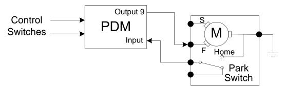
The wiper unit can be wired directly to the PDM as long as it is only connected to one output.
