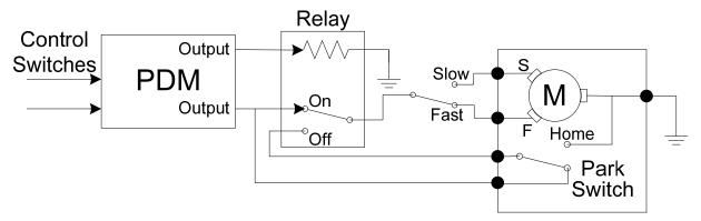
The two switch method can be modified for intermittent operation by replacing the on/off switch with a relay. The PDM controls the relay to perform the intermittent function. This requires two PDM outputs; one to supply power and the other to control the relay.
