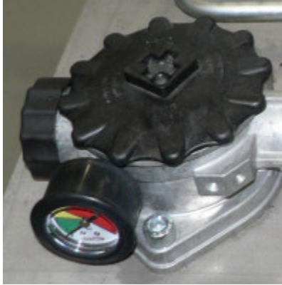
Figure 13. Fill the oil tank through the return oil filter cap
