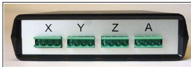
Rear pannel of boxed cobra board, with header for detachable screw terminals
