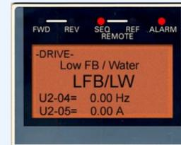
The feedback level has dropped below P1-07 for the time specified in P1-08 or Low Water input is active. Low feedback fault is active in Auto Mode when the iQpump is running.
