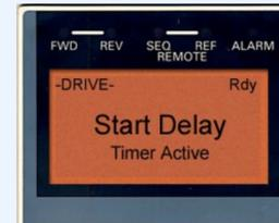
Displays when the iQpump is about to start. The feedback level has fallen below the Start Level (P1-04) and the start delay timer is active. Once the Start Level delay Time (P1-05) expires the iQpump will start.
