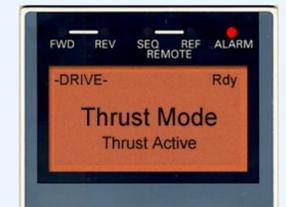
Displays when "Thrust Bearing" mode is active. To enable, enter value in parameter P4-05.
