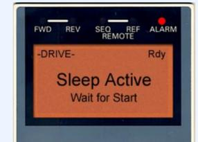
Displays when the iQpump is in "sleep" mode or when the iQpump is waiting for the feedback level to drop below the Start Level (P1-04).
