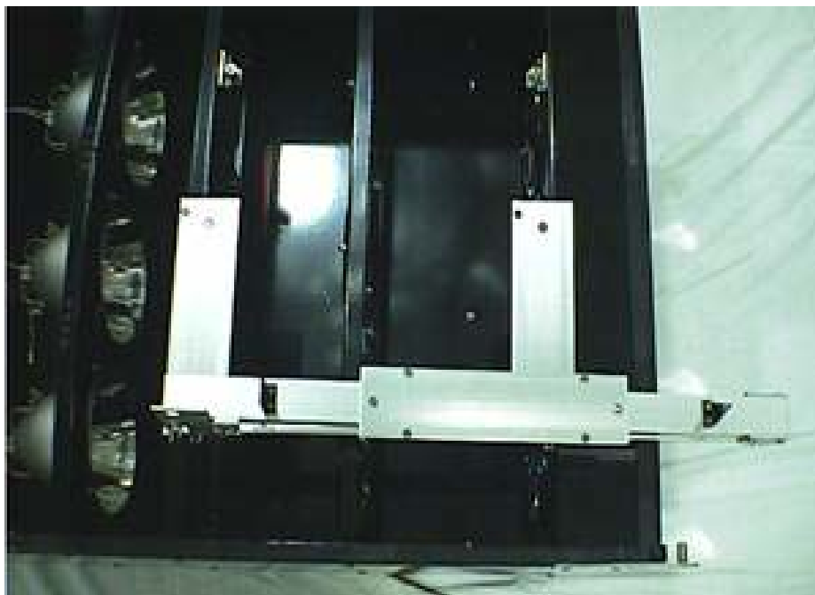
Figure 13: Top View of Bubble-Level Aiming Device for Three-Lamp PAPI
